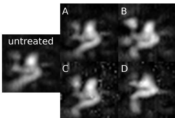
Figure 3: Maximum projections of mean contrast filling of the models during bolus injection. Untreated aneurysm model (left) and models treated with Medina devices (A, B), flow diverting stent (C), and stent assisted coiling (D).
