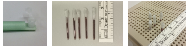
Figure 1: Picture of a delta sample mounted on the calibration rod (left) and the used glass capillaries filled with ferucarbotran (middle) that are mounted on a patch panel to setup the resolution phantom (right). The distances between the capillaries in both directions are 4.3 mm and 7.3 mm.
