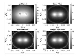
**Figure 3:** Reconstructed images of two dots 1x1 mm<sup>2</sup> separated by 7 mm: Unfiltered, Hann, Ram-Lak and Shepp-Logan filters for 41 FFL-translations and 18 projections
