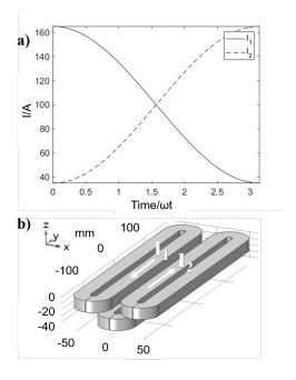
**Figure 2:** a) Current patterns applied to the selection coils. b) Coil system used in simulations. Upper and lower coils generate selection and drive fields, respectively.
