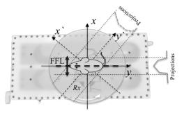
**Figure 1:** Single-sided MPI scanner. The FFL is generated through the selection coils along the y axis and translated along x axis while the subject turntable is mechanically rotated.
