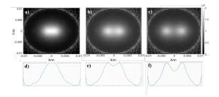
**Figure 4:** Reconstructed images using the Ram-Lak filter with 41 FFL-translations, 18 projections and a distance between the two SPIONs of (a) 3, (b) 5, and (c) 7 mm. The corresponding cross sections profiles are: (d) 3, (e) 5, and (f) 7 mm.
