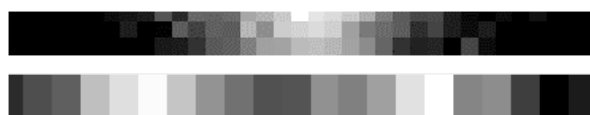
Figure 3: (top) Bottom-half of the 2-dimensional point-spread-function (PSF) of the gridded signal, (bottom) 1-dimensional relaxation MPI image of two point samples (at 10 mm distance). Length of the field-of-view (FOV) is 20 mm in both images.
