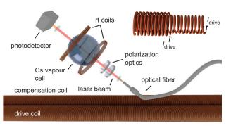
**Figure 1:** Experimental set-up of the OPM-based MPS. Top right inset: Current flow in the two (opposite handedness) layers in one of the two identical double-layered solenoids. The currents flow in opposite directions in the second double solenoid.
