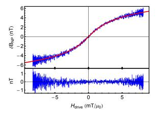
**Figure 2:** Typical  $\delta B_{\rm NP}(H_{\rm drive})$  response of a 0.5 ml Ferrotec EMG–707 sample containing 0.3 mg of iron. The data, representing 50 averaged sinusoidal  $H_{\rm drive}(t)$  cycles (total recording time of ~5 s) are fitted by Eq. 8. The lower graph shows the fit residuals.
