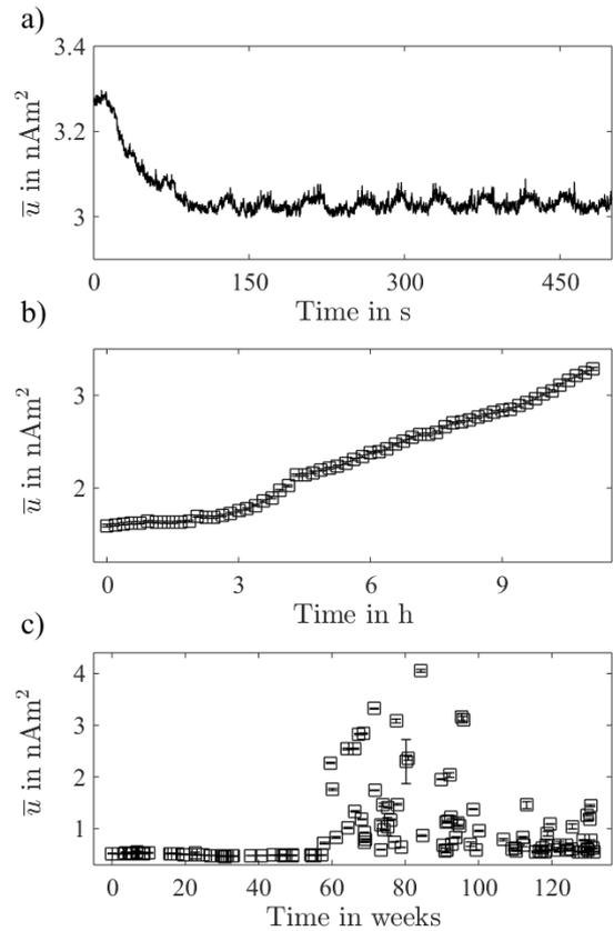
**Figure 2:** Signal deviation of the mean MPI signal amplitude in the short- (a), mid- (b) and long-term (c) regime respectively. b) and c) display mean values with the standard deviation presented as error bars.
