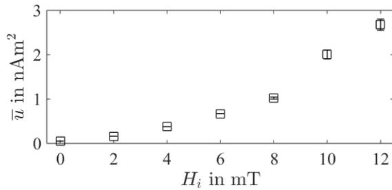
**Figure 1:** Mean MPI signal amplitude as a function of drive field amplitude. Displayed are mean values with the standard deviation presented as error bars.
