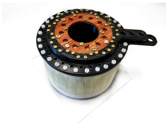
Figure 4: Assembled Halbach system consisting of two quadrupoles and one dipole with a 5.5 cm hole in the center and handles for easy rotation of the outer rings.
