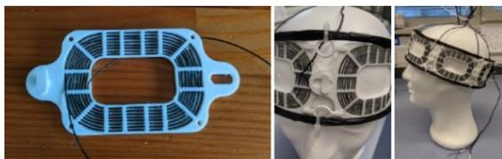
**Figure 2:** Left: Single flat coil made of highly flexible material. Middle&Right: Headband consisting of six individual flat coils for each brain area and two additional solenoids fitting around the head.
