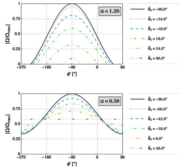
**Figure 2:** Angular velocity  $\Omega$  of MNPs for different starting angles in the respective local frame of reference. Upper row exemplary for a lock case and lower row exemplary for a drift case value of  $\alpha$ . Please note that in the local frame of reference for the lock case the phase angle depends on the chosen trajectory represented by  $\tilde{\theta}_0$ .
