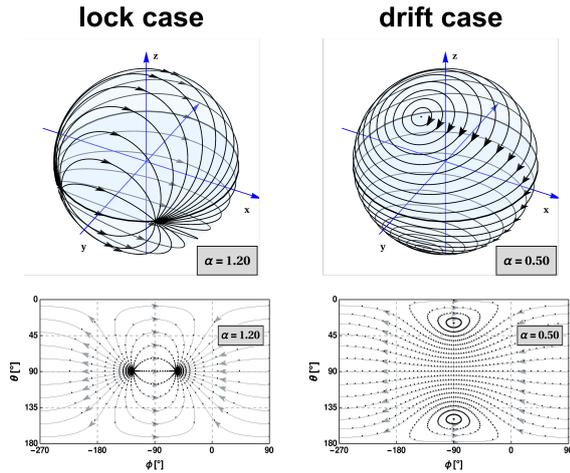
**Figure 1:** Exemplary trajectories of the MNP magnetization. The upper row shows the 3-D motion in the rotating frame of reference when the magnetic field axis points along the x-direction. In the lower row the same motion is shown in polar and azimuthal angle coordinates. The parameter  $\alpha = mB/\xi\omega_0$  with  $\omega_0$  as the rotation frequency of the external magnetic field describes the interplay between magnetic and geometric/viscose properties of the particle/liquid.
