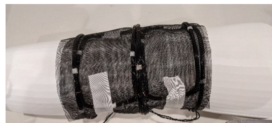
Figure 3: Example of a flexible dual-channel receive coil, which can be wrapped around the sample to increase the SNR.
