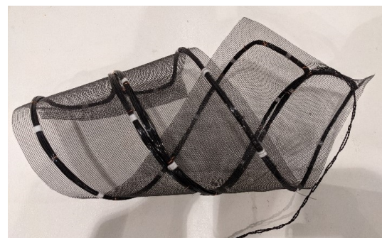
Figure 1: left: basic hardware concept for the generation of the field free line (FFL) encoding scheme. The main gradient system generates dynamically the FFL aligned into y-direction. Additional coils are used for deflection in x-z-plane for generating the projection image. Right: picture of the first iMPI prototype.
