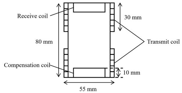
Figure 1: The structure and size of the coils of the system.
