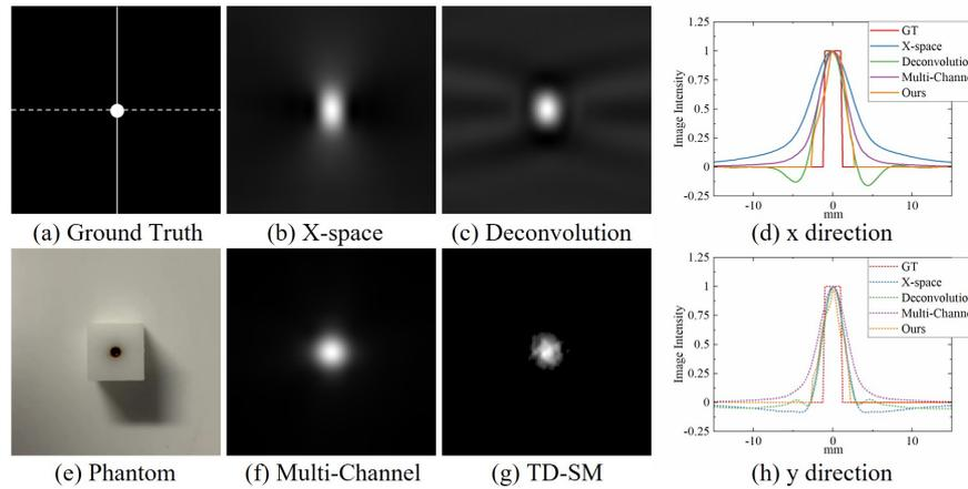
**Figure 2:** Experiment results of different reconstruction methods for a circle phantom with a diameter of 2mm.
