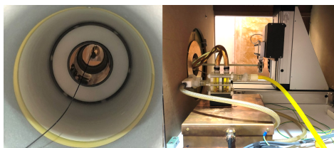
Figure 2: Hyperthermia insert and the impedance matching network integrated in the MPI scanner. Left: the hyperthermia insert installed in the scanner bore seen from the bore opening side of the scanner. Right: the impedance matching network placed beside the robot with the cooling connections.
