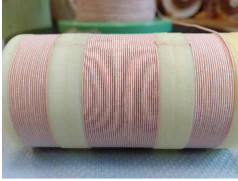
Figure 4: Second order magnetic gradiometer with a center coil and two compensation coils on the left hand and right hand side.
