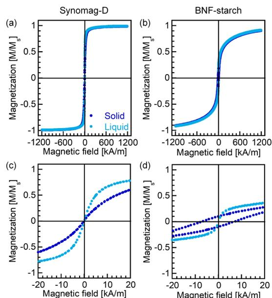
**Figure 1:** Magnetization curves under DC magnetic field of 0–1200 kA/m in (a) Synomag<sup>®</sup>-D, and (b) BNF-starch. The magnified graphs around the origin in (a) and (b) were shown in (c) and (d), respectively.
