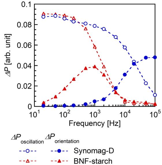
**Figure 3:** Frequency dependence of the oscillation and orientation of the easy axis under AC magnetic fields of 8 kA/m.  $\Delta P_{\text{oscillation}}$  and  $\Delta P_{\text{orientation}}$  are the degree of the oscillation and orientation of the easy axis evaluated by the optical transmission, respectively.
