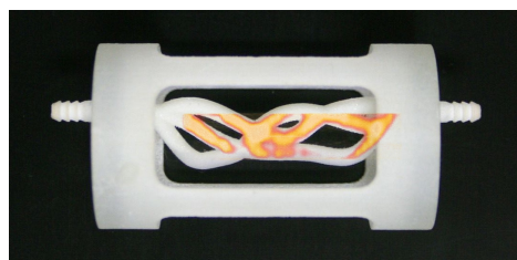
Figure 8: Realized vessel-like phantom including an overlay of one of the reconstructed images from Figure 9.
