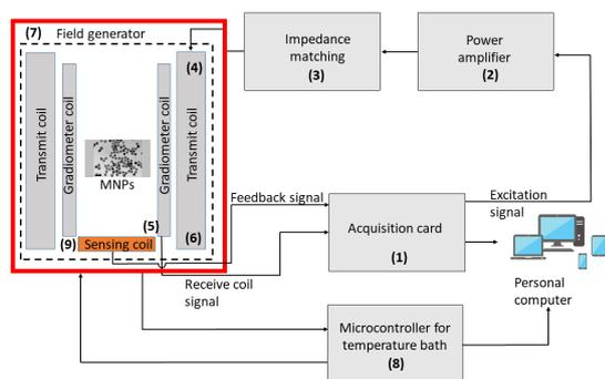
**Figure 1:** Block diagram consisting of the different modules of INSPECT
