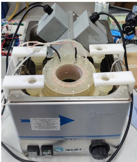
**Figure 2:** The field generator is placed inside the heating basin, which can be programmed to heat the contents inside up to user-defined temperature and duration.
