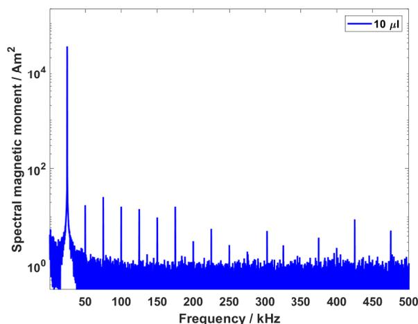
**Figure 3:** Measurements showing the sensitivity of INSPECT II using commercially available MNPs known as Resovist. The graphs show the amplitude spectrum of SPIONs for 10  $\mu\text{L}$ .
