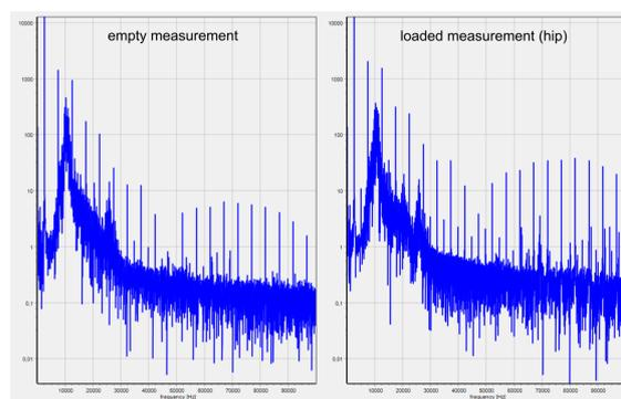
**Figure 3:** Raw spectra of an empty measurement (left) and for an experiment loaded with the hip endoprosthesis sample (right).
