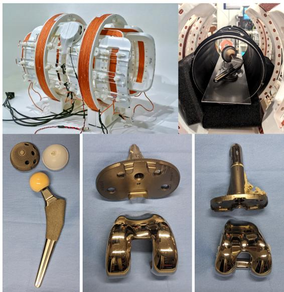
**Figure 1:** Top left: human-sized iMPI scanner for vascular intervention of the leg. Top right: photo of the experimental setup for investigating the influence of endoprosthesis on the image quality. Bottom: images of different endoprosthesis of the hip and knee.
