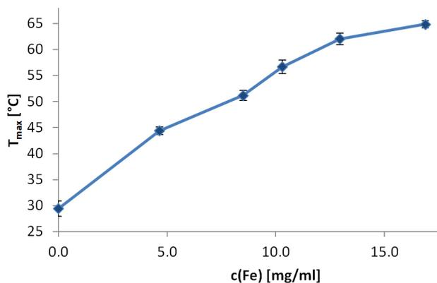
**Figure 4:** Heating profile of SEON<sup>LA-BSA</sup> in dependence of the iron content [10]. The maximum heating temperature  $T_{\max}$  is dependent on the concentration of the nanoparticle suspension.
