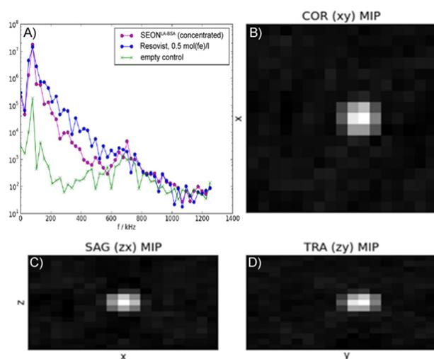
**Figure 6:** a) Comparison of the MPS signal of SEON<sup>LA</sup>-BSA-nanoparticles and Resovist<sup>TM</sup> at different frequencies. b)–d) MPI-signal of a point sample of SEON<sup>LA</sup>-BSA-nanoparticles.
