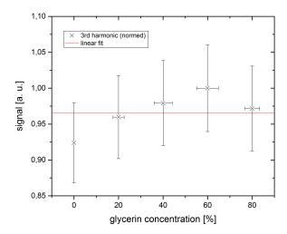
**Figure 2:** Measured signal for the same amount of particle solution mixed with different glycerin/water solutions resulting in a glycerin content from 0 % to 80 %.
