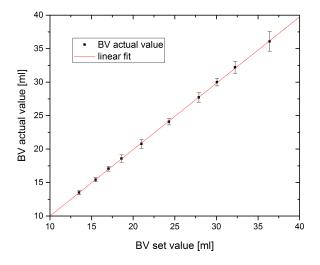
**Figure 3:** The measured total circulating blood volume (BV actual value) versus the given total circulating blood volume (BV set value). The linear fit is shown in red.
