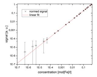
**Figure 1**: Measured Signal of the third harmonic versus the concentration of FeraSpin<sup>TM</sup> R. The error bars represent both the measurement uncertainty and a pipette error of 2%.
