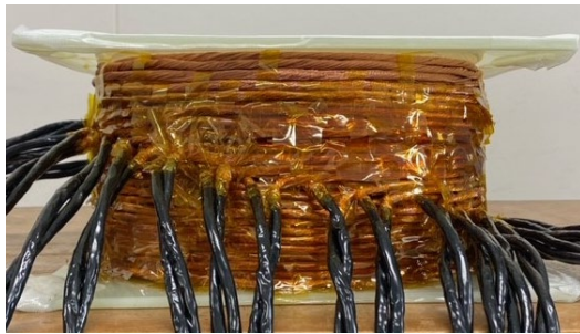
Figure 2: Drive field coil made of Cu Lits-wire.
