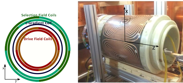
Figure 1: The field generator of the rabbit-sized FFL scanner. Left: It consists of two pairs of drive field coils (red), a Maxwell coil (blue) and two pairs of selection field quadrupole coils (green). Right: The realized setup at which the outermost quadrupole coil can be seen.
