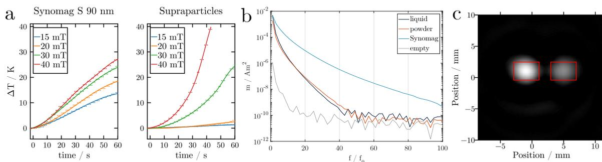
**Figure 1:** **a)** temperature increase during hyperthermia experiment at 300 kHz using different amplitudes, **b)** MPS spectra (odd harmonics) comparing the supraparticles with Synomag, **c)** MPI image of powder supraparticles samples at 1.1 mm distance
