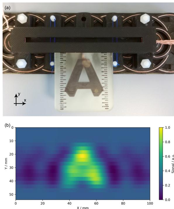
**Figure 1:** a) The prototype of 10 channel 1D MPI system and b) a reconstructed image of the sample. The position of the encoding line roughly coincides with the visible slot in the drive field coil.
