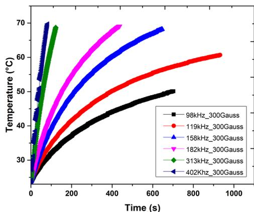
**Figure 1:** Calorimetry measurements at 300 G applied AMF demonstrate increase in heating rate with frequency.
