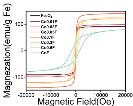
**Figure 1:** Magnetization curves (M-H) of  $\text{Co}_x\text{Fe}_{3-x}\text{O}_4$  MNPs at 300 K.
