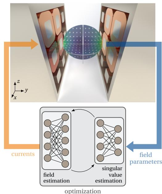
**Figure 1:** A schematic representation of field control is shown. The upper section depicts the coil array with soft iron cores. The 8 coils utilized in this study are highlighted. An exemplary generated field is situated in the center. At the bottom, the optimization process is illustrated. An optimizer adjusts the currents based on optimization goals and constraints, employing neural networks for both field and gradient prediction.
